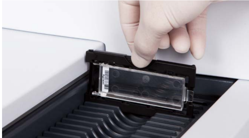
Figure 44 Inserting slide holder into cassette
