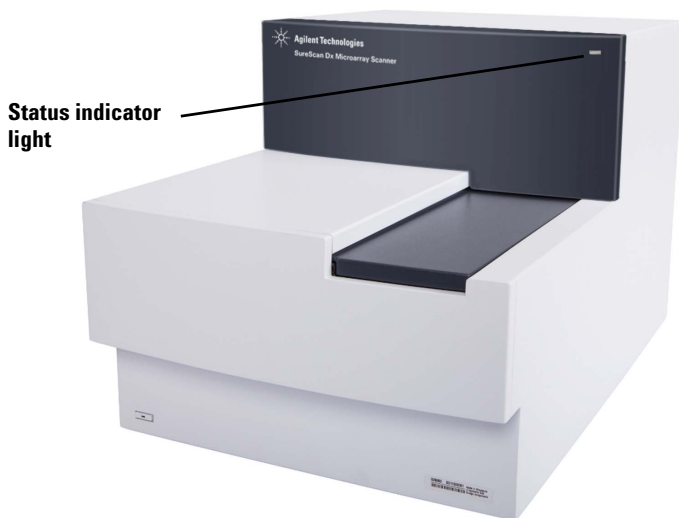
Figure 13 Location of the status indicator light
