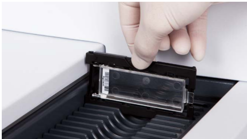
Figure 12 Inserting slide holder into cassette
