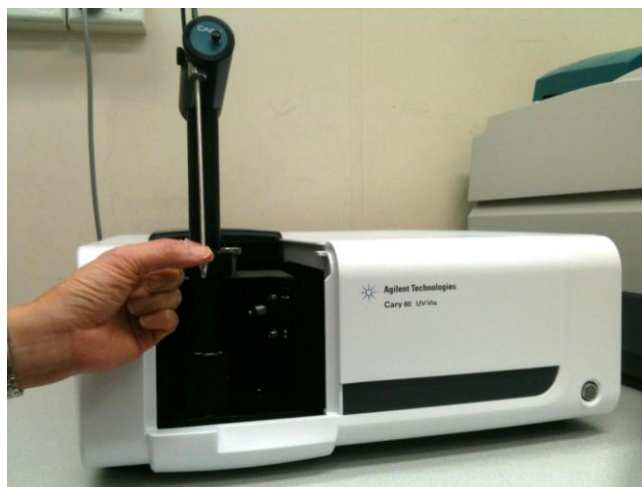
Figure 1. The Cary 60 instrument fitted with the Fiber Optics Accessory taking a reading of 50 µl DNA in an Eppendorf tube at 4 °C
