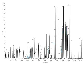
**Total Ion Chromatogram of EPA Method 524.2 ICAL standard,** acquired using the GC, MSD, and P&T parameters contained in Agilent's GC/MS VOC Application Kit. Excellent stability, robustness, and peak shape were achieved – and detection limits were lowered to PPB or PPT levels.
