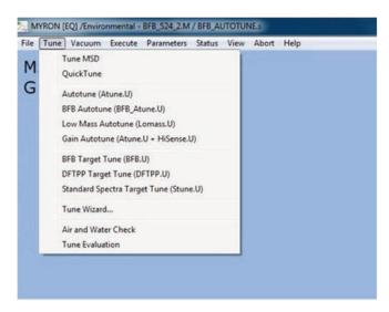
Tune and vacuum control view of the Agilent MSD Productivity ChemStation. BFB Autotuning provides long-term stability and improves sensitivity into the PPT range.
