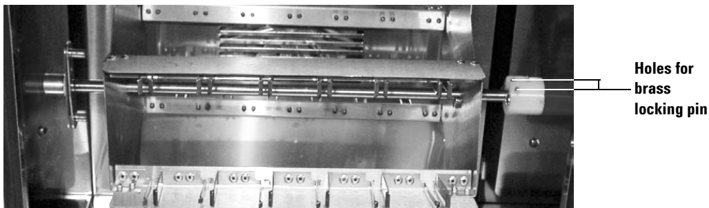
Figure 5 Rotator correctly installed
