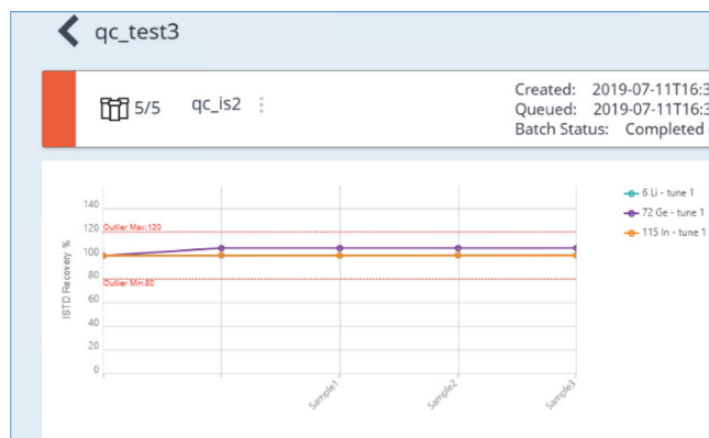
Figure 1. ICP Go screen showing ISTD recovery plot with high and low limits.
