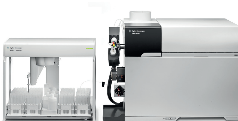
Figure 1. Agilent 7900 fitted with the optional ISIS 3 discrete sampling (DS) accessory and coupled to an Agilent SPS 4 autosampler
