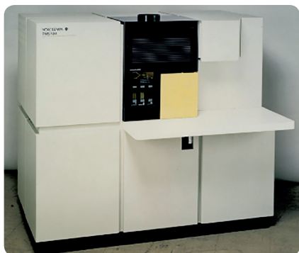
PMS100: First commercial ICP-MS with off-axis lens, hyperbolic quadrupole, and computer control (1987).
