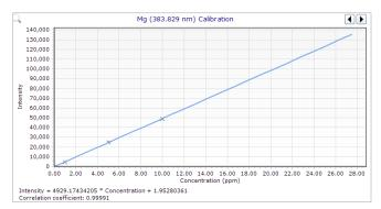
Figure 1. Calibration curve for Mg 383.829 nm
