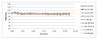
Figure 2. Long-term stability plot. <2.0% RSD over 12 hours analysis of river sediment sample
