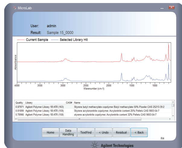
Figure 4a (top), 4b (bottom). After analyzing an unknown sample, Agilent MicroLab software searches the on-board spectral database for best match. The spectrum and identity of the unknown sample is displayed as is the spectrum of its best library match and a numerical value reflecting the quality of the match.
