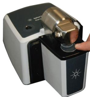
Using the TumbIR to measure thin polymer films eliminates the need to mount samples on a card. This allows you to see exactly where in the sample you are measuring as well as eliminating fringe patterns on the film. DialPath shown here.
