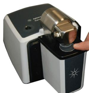
Using the DialPath to measure thin polymer films eliminates the need to mount samples on a card. This allows you to see exactly where in the sample you are measuring as well as eliminating fringe patterns on the film.
