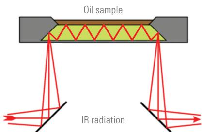
Optical diagram of the Agilent 5 bounce ZnSe ATR accessory
