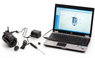
Redefining Mechanical Qualification, the 280-DS Mechanical Qualification System provides quantitative values for all physical parameters of the dissolution apparatus. It is designed to take quick, accurate measurements at the proper locations as prescribed by current industry regulations.
