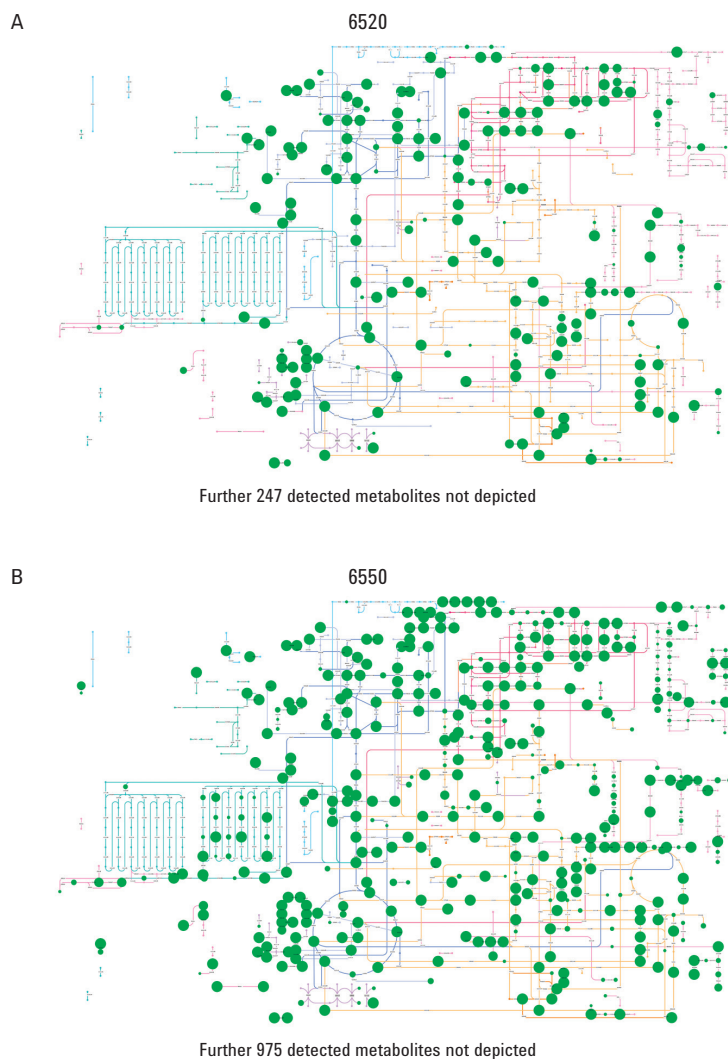
Figure 3. This map reports the compounds found by annotation and demonstrates six to seven times greater coverage with the Agilent 6550 Q-TOF (B) as compared to the 6520 Q-TOF (A). Dot sizes scale with the degree of confidence for the annotation.
