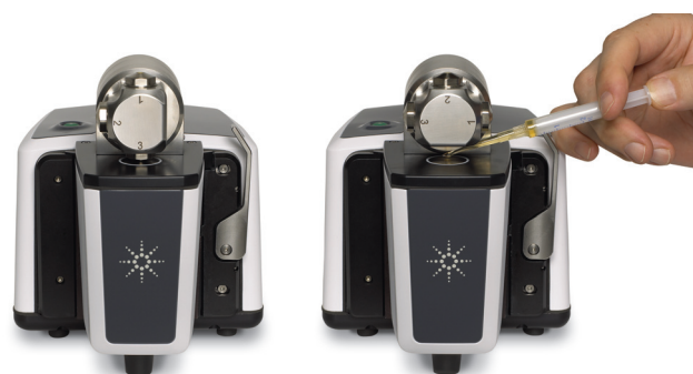
Figure 2. DialPath technology allows users to change between three factory-calibrated, fixed pathlength selections in seconds
