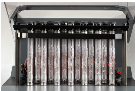
A set of 13 dissolution cells surrounded by heating jackets and situated on top of a sampling port provide a high level of automation, throughput and convenience.
