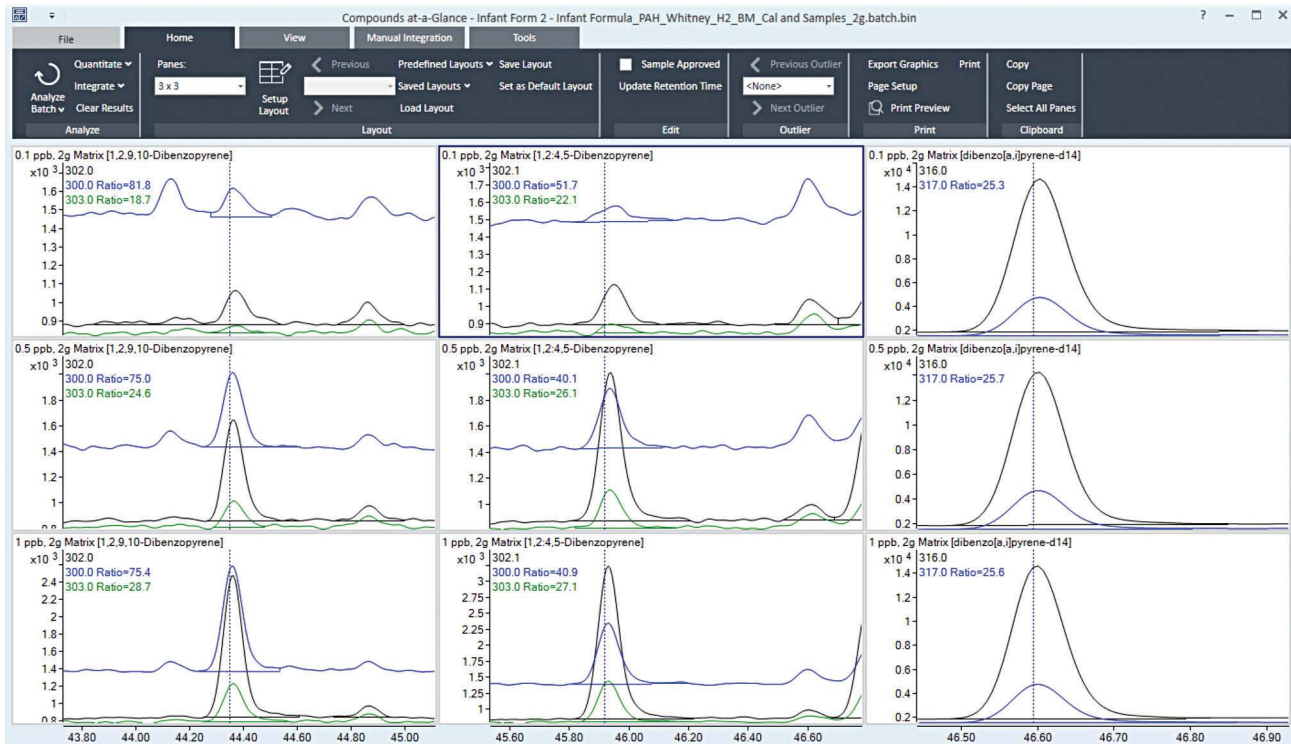
Highly customizable Compounds-at-a-Glance view for 1,2,9,10-dibenzopyrene, 1,2,4,5-dibenzopyrene, and dibenzo[a,i]pyrene-d14 at 0.1, 0.5, 1, calibration levels.
