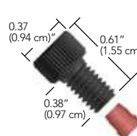
P-945x 2 Delrin Nut, M6 with P-940 Ferrule
