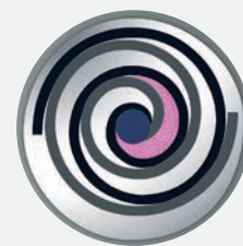
Gas exhausted at center hub
