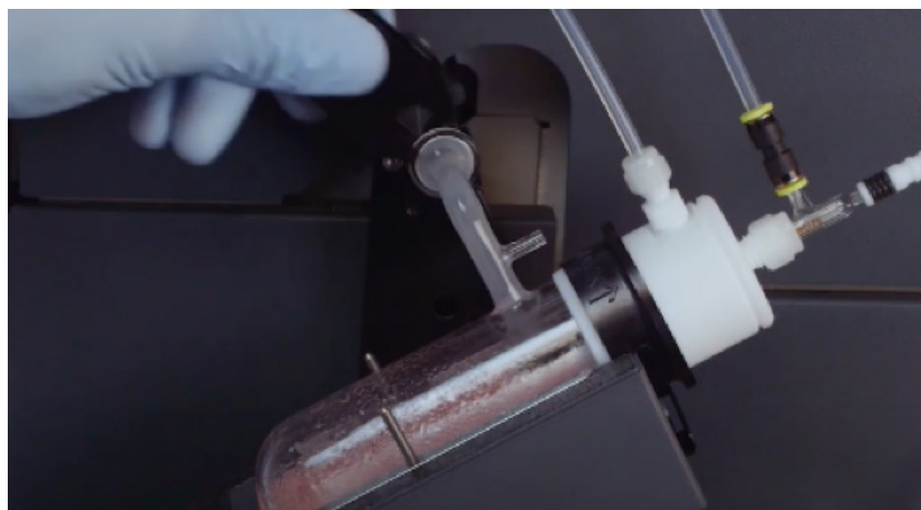
Excessive droplet formation inside the spray chamber is one of the signs that the spray chamber may require cleaning.
